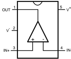
**Figure 2. 5-Pin SOT-23 (Top View)**
