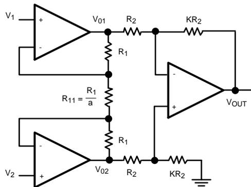
Figure 50. Instrumentation Amplifier
