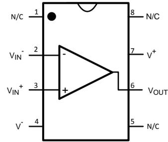
**Figure 3. 8-Pin SOIC (Top View)**
