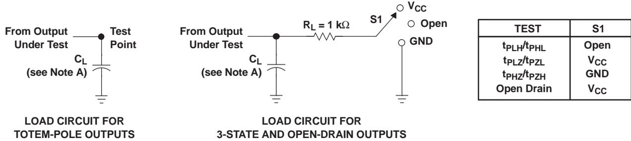
LOAD CIRCUIT FOR TOTEM-POLE OUTPUTS
