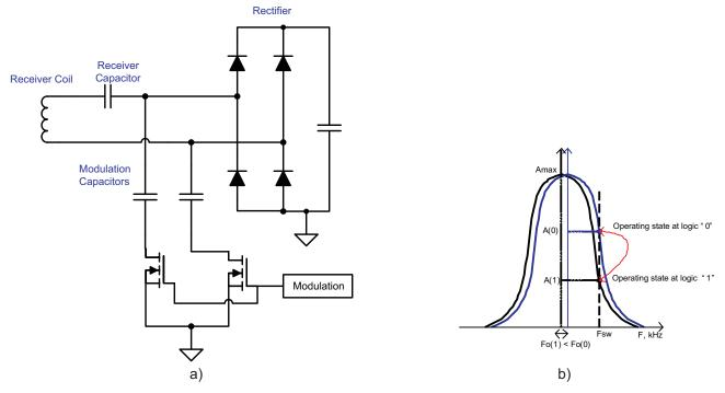
Figure 4. Capacitive Modulation Circuit
