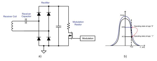
Figure 3. Resistive Modulation Circuit
