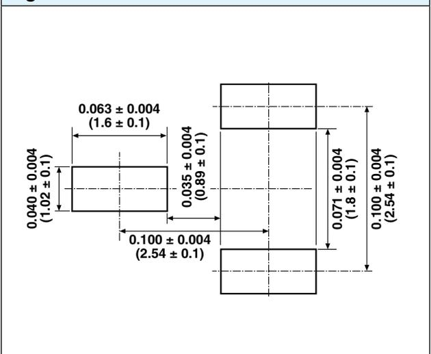
Figure 6 – Dimensions and Imprinting
