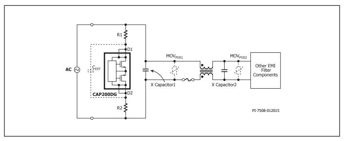
Figure 4. Placement Options of MOV and C<sub>FXT</sub>\*
