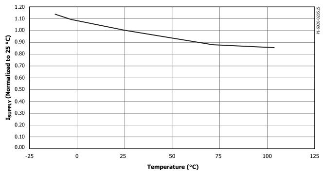
Figure 6.  $I_{SUPPLY}$  vs. Temperature.
