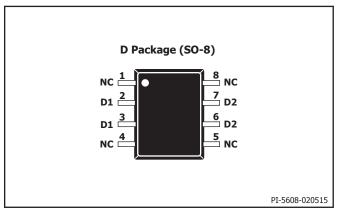
Figure 3. Pin Configuration.
