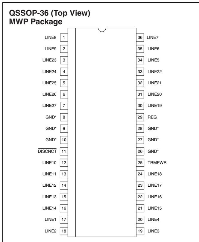
\* MWP package pins 8 - 10 and 26 - 28 serve as heatsink/ground.
