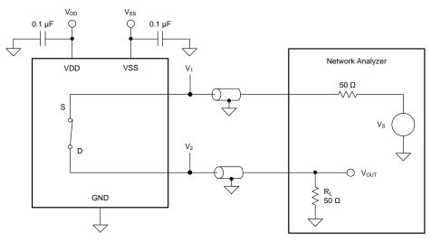
Figure 36. Bandwidth Measurement Setup
