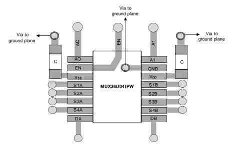
Figure 47. MUX36D04IPW Layout Example
