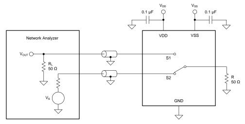
Figure 35. Channel-to-Channel Crosstalk Measurement Setup
