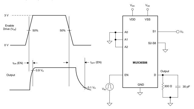
Figure 32. Turn-On and Turn-Off Time Measurement Setup
