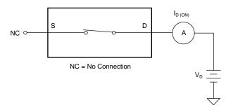
Figure 28. On-Leakage Measurement Setup
