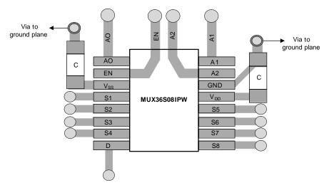
Figure 46. MUX36S08IPW Layout Example
