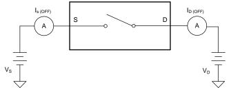
Figure 27. Off-Leakage Measurement Setup
