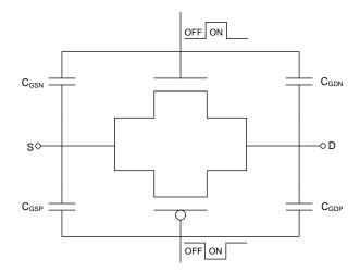
Figure 39. Transmission Gate Topology
