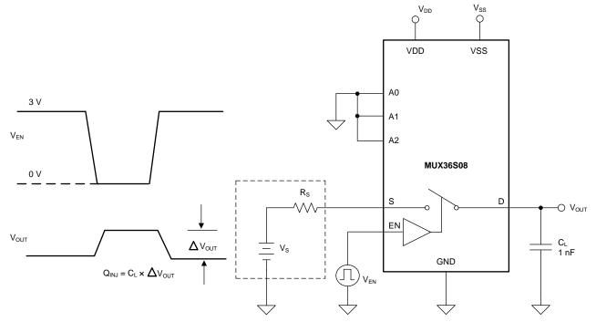
Figure 33. Charge-Injection Measurement Setup
