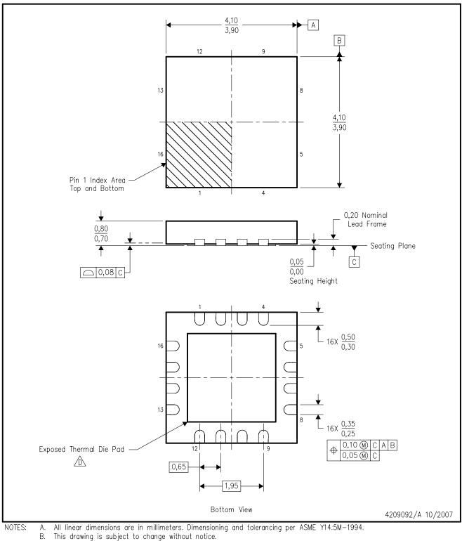
C. QFN (Quad Flatpack No-Lead) package configuration.
