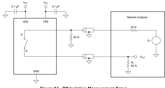
Figure 34. Off Isolation Measurement Setup
