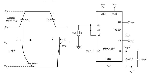
Figure 30. Transition-Time Measurement Setup
