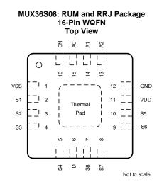
RUM and RRJ have the same package dimension, but different thermal pad dimension and lead finger length.
