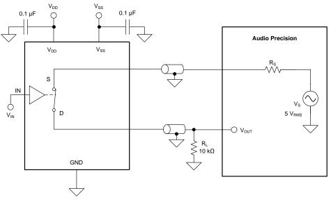
Figure 37. THD+N Measurement Setup
