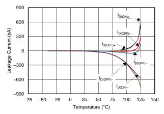
Figure 38. Leakage Current vs Temperature
