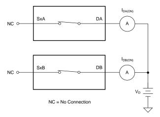
Figure 29. Differential On-Leakage Measurement Setup
