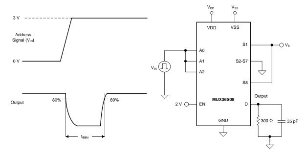
Figure 31. Break-Before-Make Delay Measurement Setup
