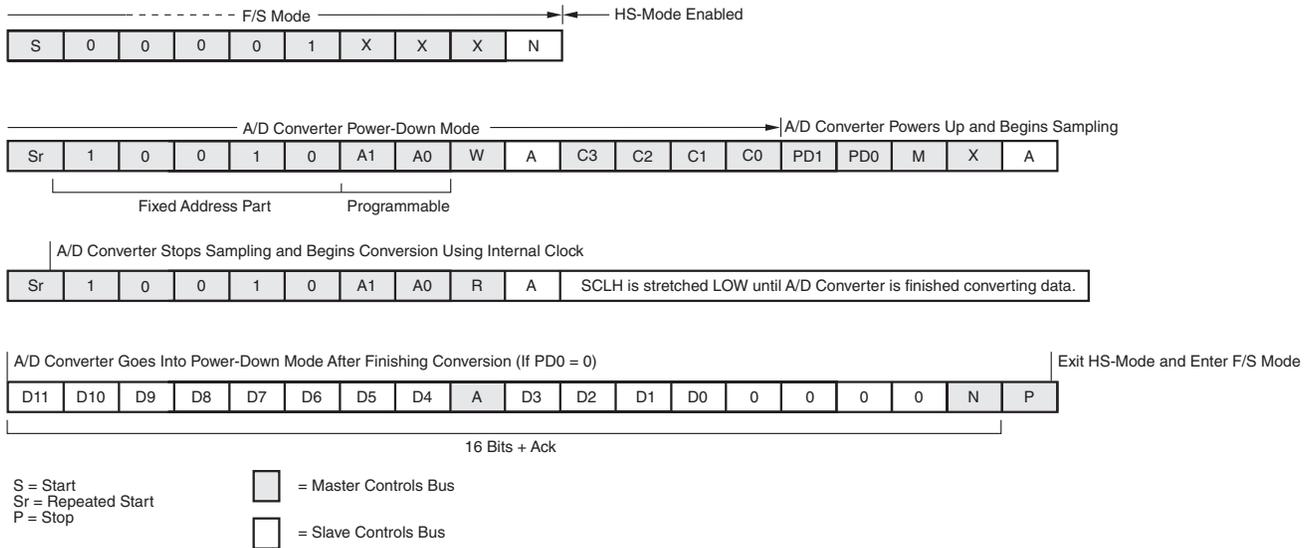
Figure 16. High-Speed I<sup>2</sup>C Mode Conversion Cycle
