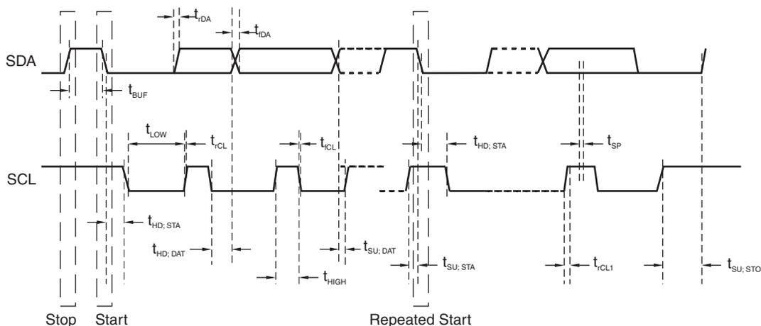
Figure 1. Timing Diagram
