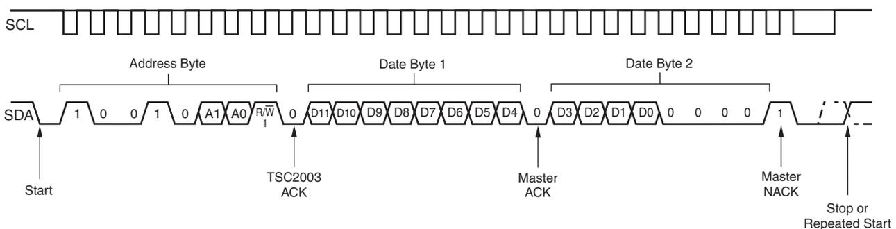
Figure 15. Complete I<sup>2</sup>C Serial Read Transmission
