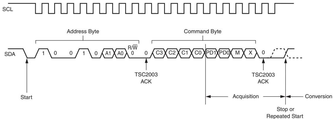
Figure 14. Complete I<sup>2</sup>C Serial Write Transmission
