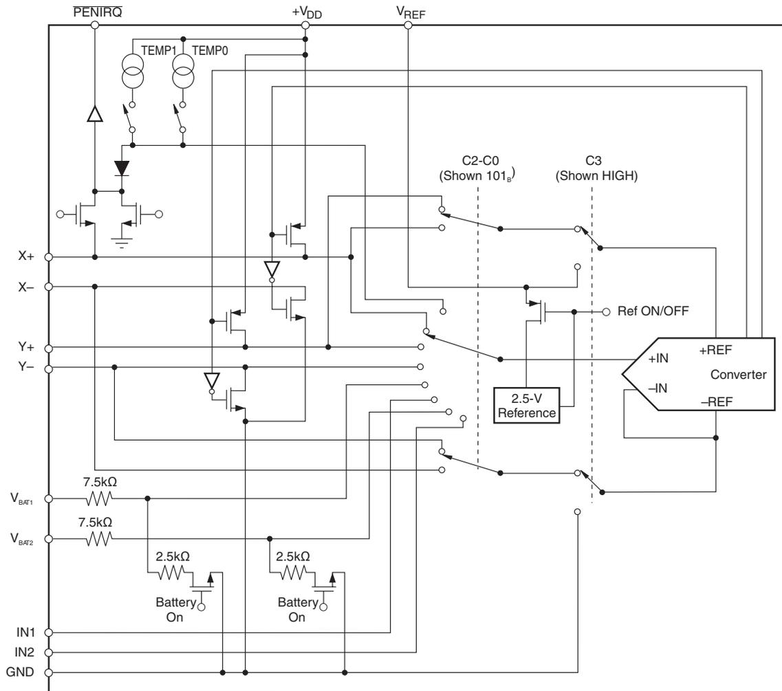
Figure 4. Simplified Diagram of the Analog Input
