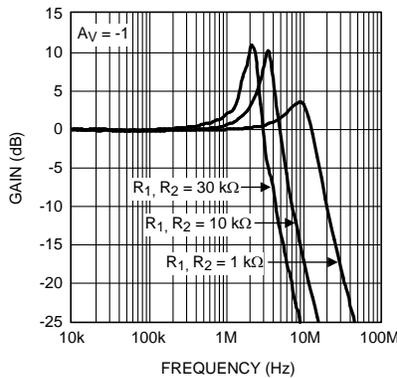
Figure 47. Gain Peaking Caused by Large  $R_1$ ,  $R_2$
