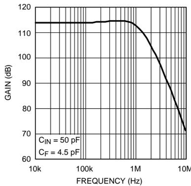
Figure 58. 1.5 MHz Transimpedance Amplifier Frequency Response
