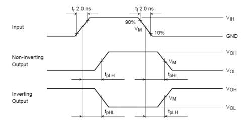
Fig. 12.8.1 t<sub>PLH</sub>, t<sub>PHL</sub>
