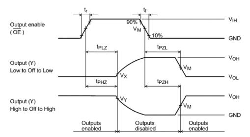
Fig. 12.8.2 t<sub>PLZ</sub>, t<sub>PHZ</sub>, t<sub>PZL</sub>, t<sub>PZH</sub>
