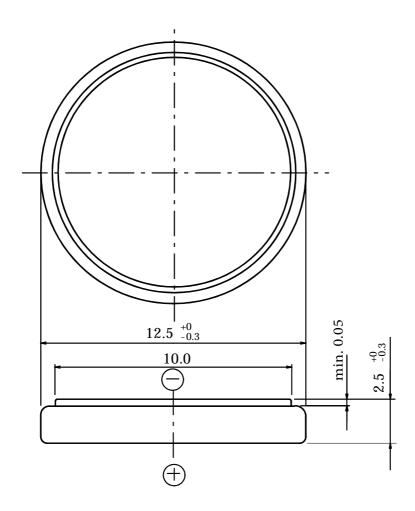
Terminal : Plus terminal material : Minus terminal material : Nickel plated Stainless steel Nickel plated Stainless steel
