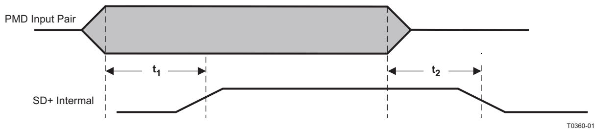
Figure 9-20. 100Base-TX Signal Detect Timing
