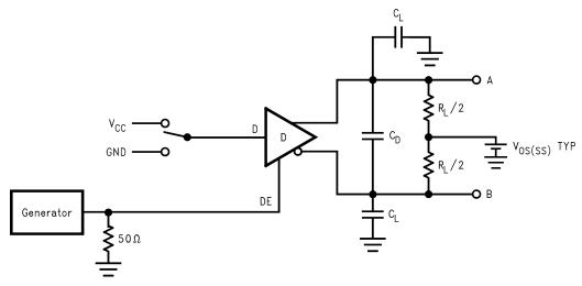
Figure 8. Driver TRI-STATE Delay Test Circuit
