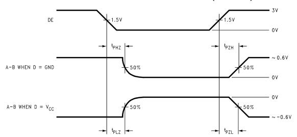
Figure 9. Driver TRI-STATE Delay Waveforms
