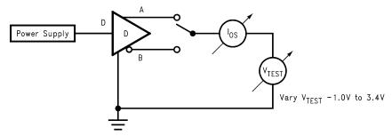
Figure 5. Differential Driver Short-Circuit Test Circuit
