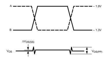
Figure 2. Differential Driver Waveforms
