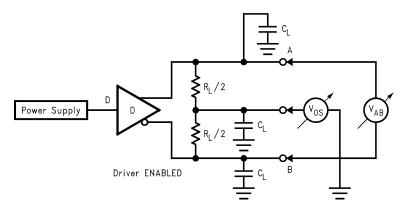
Figure 1. Differential Driver Test Circuit
