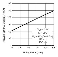
Figure 15. Driver Power Supply Current as a Function of Frequency
