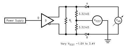
Figure 3. Differential Driver Full Load Test Circuit
