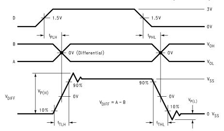
Figure 7. Driver Propagation Delay and Transition Time Waveforms
