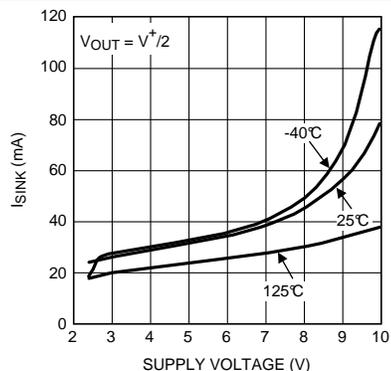
Figure 24. Sinking Current vs Supply Voltage
