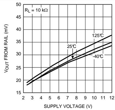
Figure 34. Output Swing Low and Supply Voltage
