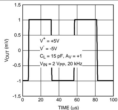
Figure 28. Large-Signal Transient
