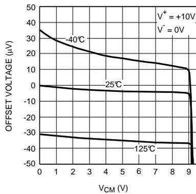
Figure 5. Offset Voltage vs  $V_{CM}$
