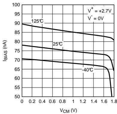
Figure 11. Input Bias Current vs  $V_{CM}$
