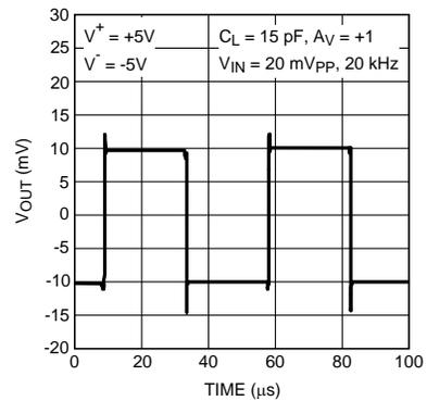
Figure 30. Small-Signal Transient Response
