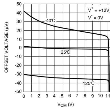
Figure 6. Offset Voltage vs  $V_{CM}$
