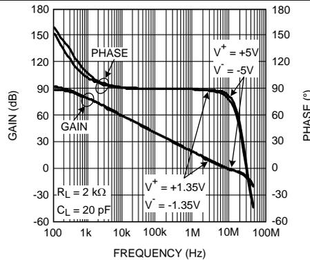
Figure 16. Open-Loop Gain and Phase With Supply Voltage
