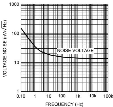
Figure 17. Input Referred Noise Voltage vs Frequency
