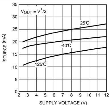
Figure 23. Sourcing Current vs Supply Voltage
