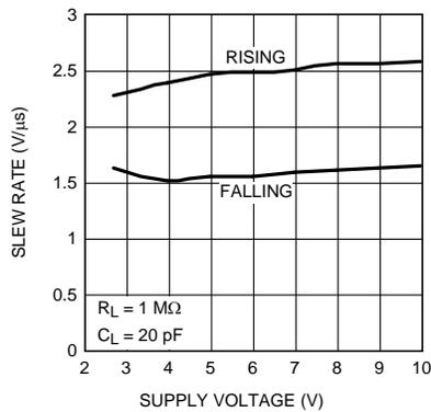
Figure 35. Slew Rate vs Supply Voltage
