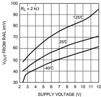
Figure 31. Output Swing High vs Supply Voltage
