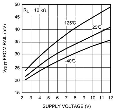
Figure 33. Output Swing High vs Supply Voltage
