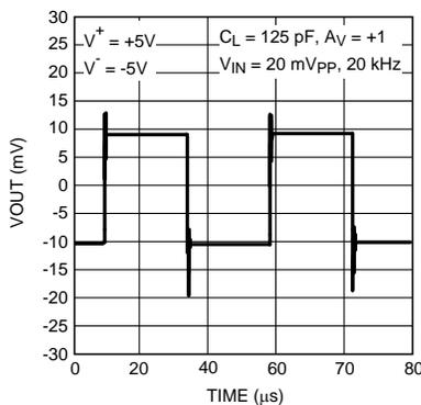
Figure 29. Small-Signal Transient Response
