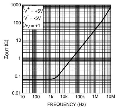
Figure 18. Close Loop Output Impedance vs Frequency
