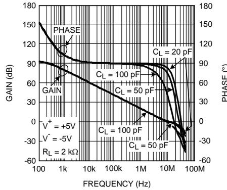
Figure 14. Open-Loop Gain and Phase With Capacitive Load
