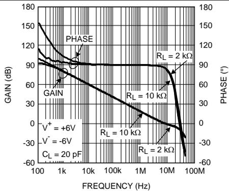
Figure 15. Open-Loop Gain and Phase With Resistive Load
