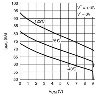
Figure 12. Input Bias Current vs  $V_{CM}$
