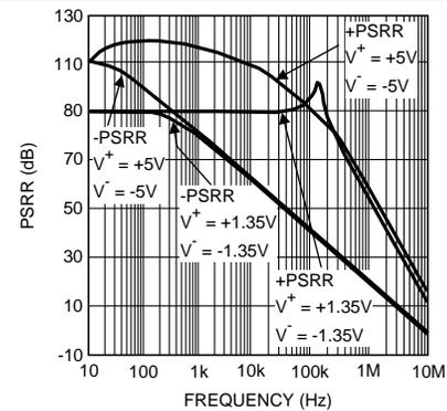
Figure 10. PSRR vs Frequency
