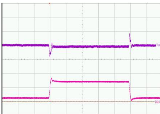
(VIN = 5 V, VOUT = 1.05 V, IOULT = 0.5 A to 3.0 A) Upper Trace: Output Voltage, 50 mV / div Lower Trace: Output Current, 2 A / div Time = 200 \mu s/div
