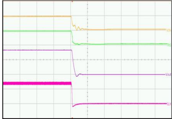
(VIN = 5 V, VOUT = 1.8 V, IOU T = 3 A) Upper Trace: Input Voltage, 5 V / div Second Trace: Power Good Pin Voltage, 5 V / div Third Trace: Output Voltage, 2 V / div Lower Trace: Inductor Current, 2 A / div Time = 200 μs / div
