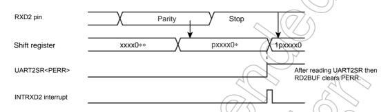
Figure 13-5 Generation of Parity Error
