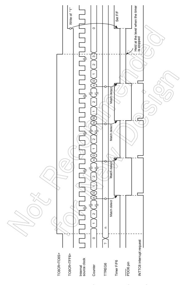
Figure 11-4 8-Bit PDO Mode Timing Chart (TC6)
