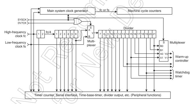
Figure 2-4 Configuration of Timing Generator
