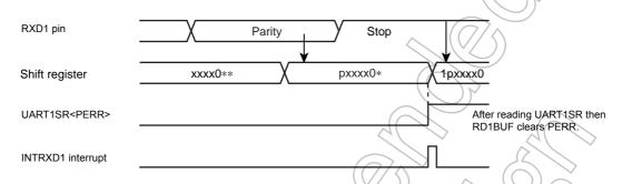
Figure 12-5 Generation of Parity Error
