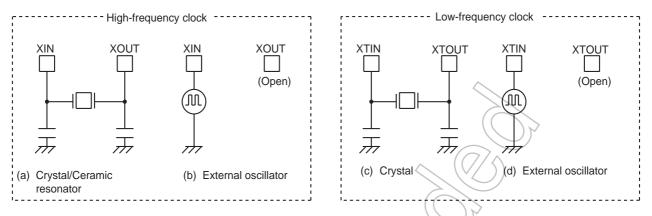
Figure 2-3 Examples of Resonator Connection
