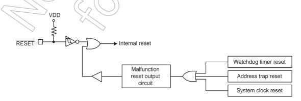
Figure 2-15 Reset Circuit
