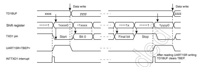
Figure 12-9 Generation of Transmit Data Buffer Empty
