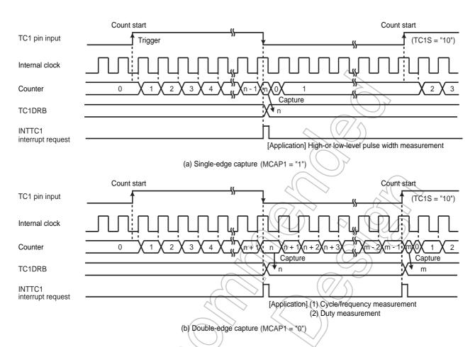
Figure 8-6 Pulse Width Measurement Mode
