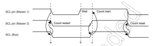
Figure 16-4 Clock Synchronization
