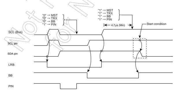
Figure 16-14 Timing Diagram when Restarting
