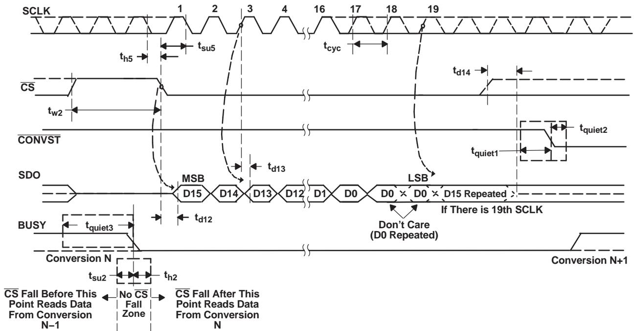
**Figure 45. Read Frame Controlled via  $\overline{CS}$  (FS = 1)**
