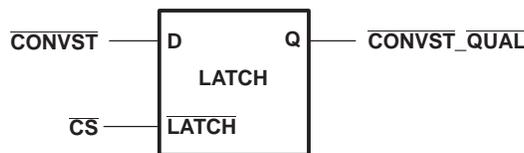
Figure 39. Relationship Between  $\overline{CONVST\_QUAL}$ ,  $\overline{CS}$ , and  $\overline{CONVST}$
