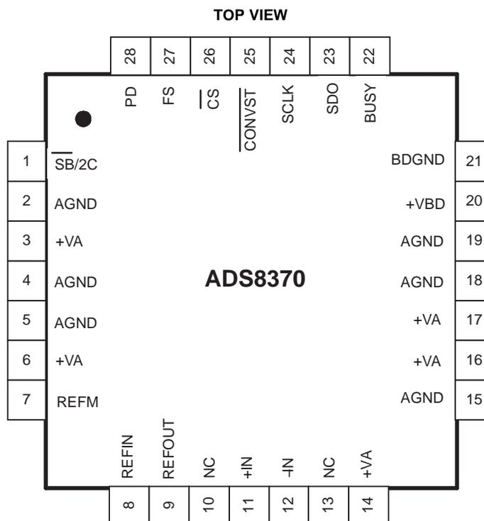
Note: The package thermal pad must be soldered to the printed circuit board for thermal and mechanical performance.
