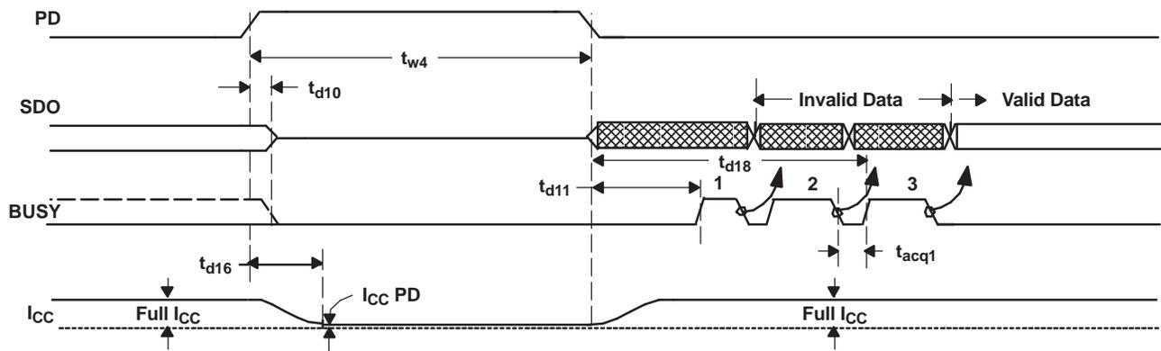
Figure 54. Device Full Power Down/Resume (External Reference Used)
