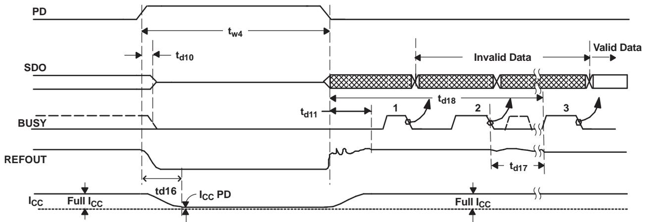
Figure 53. Device Full Power Down/Resume (Internal Reference Used)
