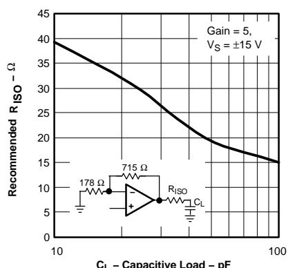
Figure 58. Recommended R<sub>ISO</sub> vs Capacitive Load
