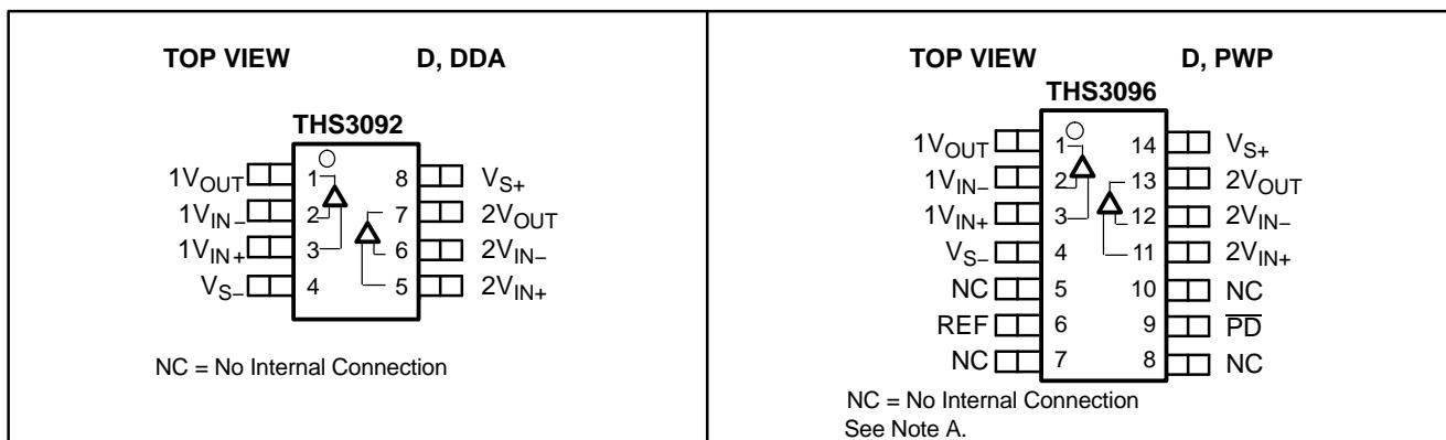
Note A: The devices with the power down option defaults to the ON state if no signal is applied to the  $\bar{P}D$  pin. Additionally, the REF pin functional range is from  $V_{S+} - 4$  V.
