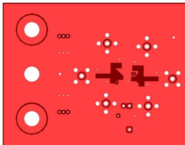
**Figure 76. THS3096 EVM Board Layout (Ground Plane)**
