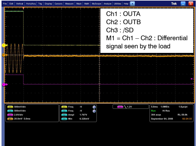
Figure 40. Zero pop noise turn off sequence with differential input audio source ( C_i = 47 \text{ nF} , R_i = 24 \text{ k}\Omega , R_f = 24 \text{ k}\Omega , C_{\text{byp}} = 1 \text{ }\mu\text{F} , R_l = 8 \text{ }\Omega , T_{\text{on}} = V_p )
