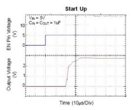
The LP3983S features an LDO regulator enable/disable function. To assure the LDO regulator will switch on, the EN turn on control level must be greater than 1.4 volts. The LDO regulator will go into the shutdown mode when the voltage on the EN pin falls below 0.4 volts. For to protecting the system, the LP3983S have a quick-discharge function. If the enable function is not needed in a specific application, it may be tied to  $V_{\text{IN}}$  to keep the LDO regulator in a continuously on state.
