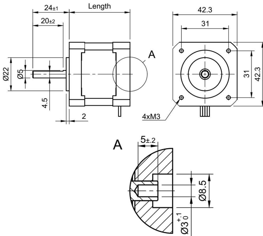
Figure 4.2: Dimensions (all values in mm)
