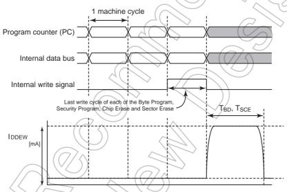
Figure 22-2 Current When an Erase or Program is Being Performed on the Flash Memory
