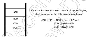
The checksum which is transmitted by executing the flash memory write command, RAM loader command, or flash memory SUM output command is calculated in the manner, as shown above.
