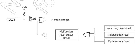
Figure 2-15 Reset Circuit
