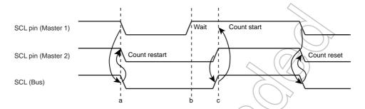
Figure 16-4 Clock Synchronization
