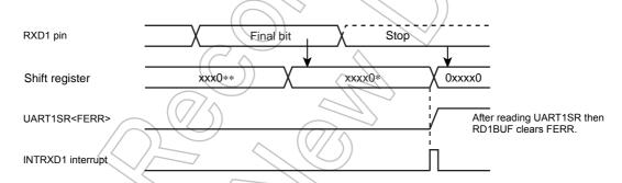
Figure 12-6 Generation of Framing Error
