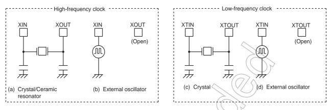
Figure 2-3 Examples of Resonator Connection
