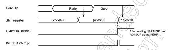
Figure 12-5 Generation of Parity Error
