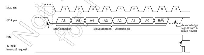
Figure 16-9 Start Condition Generation and Slave Address Transfer
