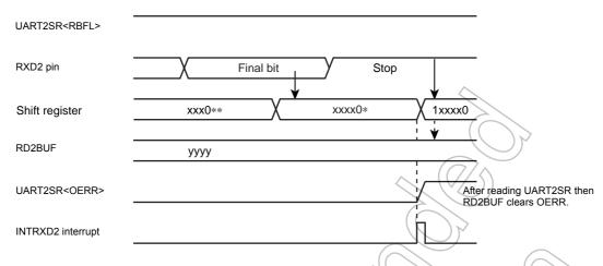
Figure 13-7 Generation of Overrun Error
