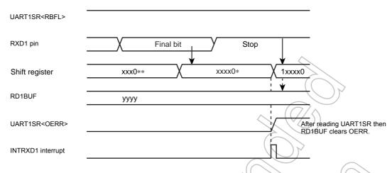
Figure 12-7 Generation of Overrun Error
