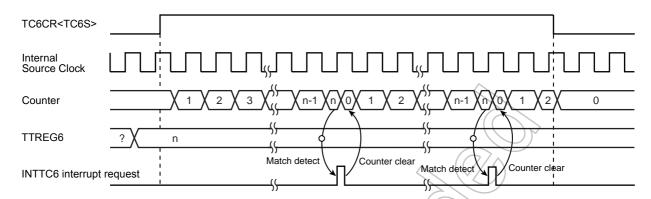
Figure 11-2 8-Bit Timer Mode Timing Chart (TC6)
