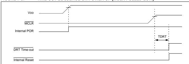
FIGURE 7-9: TIME-OUT SEQUENCE ON POWER-UP (MCLR TIED TO VDD): FAST VDD RISE TIME
