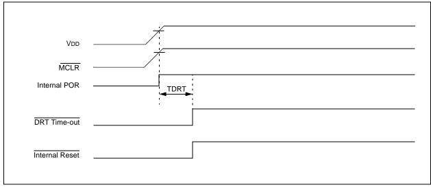
FIGURE 7-10: TIME-OUT SEQUENCE ON POWER-UP (MCLR TIED TO VDD): SLOW VDD RISE TIME
