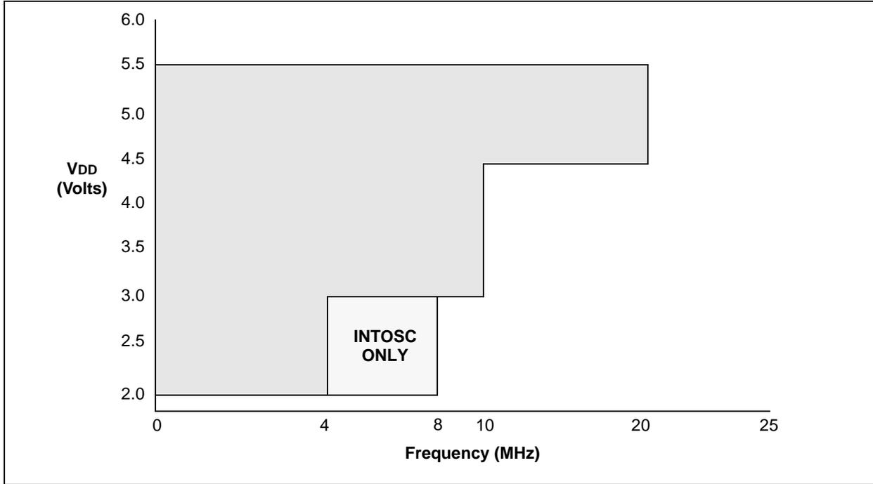
**FIGURE 11-2: MAXIMUM OSCILLATOR FREQUENCY TABLE**
