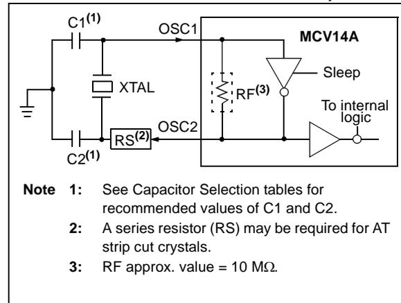
**FIGURE 7-2: EXTERNAL CLOCK INPUT OPERATION (HS, XT, LP OR EC OSC CONFIGURATION)**
