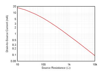
Figure 9-3. Drain-to-Source Current vs R<sub>S</sub>, V<sub>DS</sub> = 5 V
