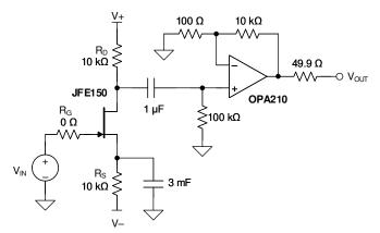
Figure 7-1. AC Measurement Reference Schematic
