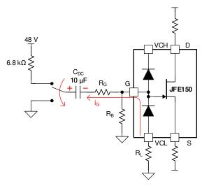
Figure 9-1. JFE150 Clamping Diode Example
