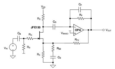
Figure 9-5. Low Noise, High Input Impedance Composite Amplifier
