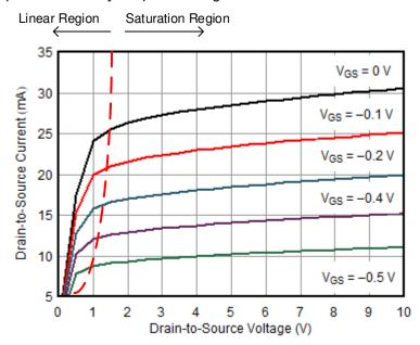
Figure 8-1. V<sub>DS</sub> vs I<sub>DS</sub>
