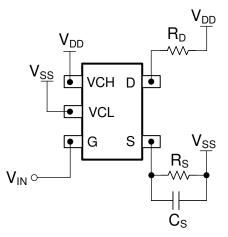
Figure 11-1. JFE150 Layout Example, Common Source Configuration
