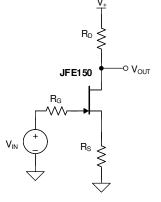
Figure 9-2. Common-Source Amplifier
