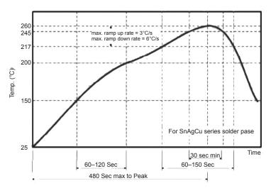
Infrared soldering profile for Chip Resistors
