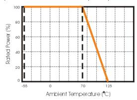
Max. dissipation in percentage of rated power as a function of the ambient temperature for MCWR08
