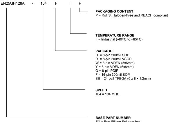
EN = Eon Silicon Solution Inc. 25QH = 3V Serial Flash with 4KB Uniform-Sector, Dual and Quad I/O 128 = 128 Megabit (16,384K x 8) A = version identifier
