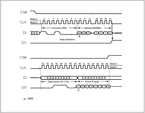
Figure 33. Read Manufacturer / Device ID Diagram
