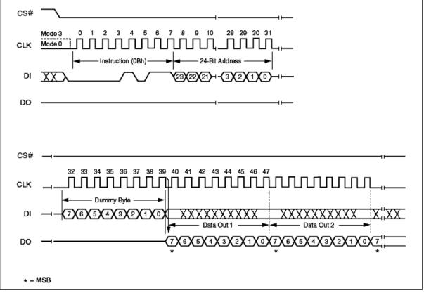
Figure 14. Fast Read Instruction Sequence Diagram
