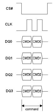
Figure 9.1 Write Enable/Disable Instruction Sequence in QPI Mode
