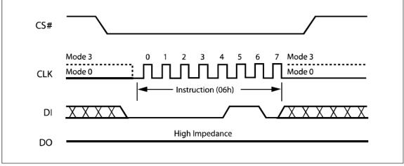
Figure 8. Write Enable Instruction Sequence Diagram
