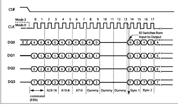
Figure 17.1. Quad Input / Output Fast Read Instruction Sequence in QPI Mode
