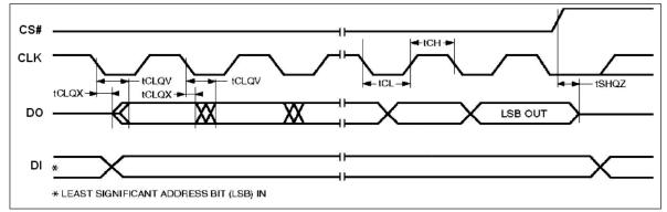
Figure 39. Serial Output Timing
