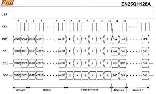
Figure 14.1 Fast Read Instruction Sequence in QPI Mode
