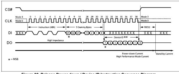
Figure 32. Release Power-down / Device ID Instruction Sequence Diagram
