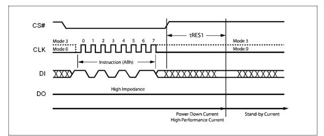
Figure 31. Release Power-down Instruction Sequence Diagram
