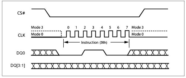
Figure 6. Enable Quad Peripheral Interface mode Sequence Diagram
