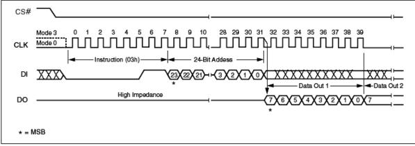
Figure 13. Read Data Instruction Sequence Diagram
