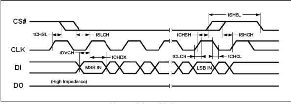
Figure 40. Input Timing
