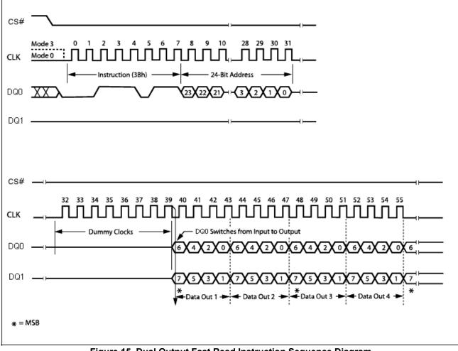
Figure 15. Dual Output Fast Read Instruction Sequence Diagram
