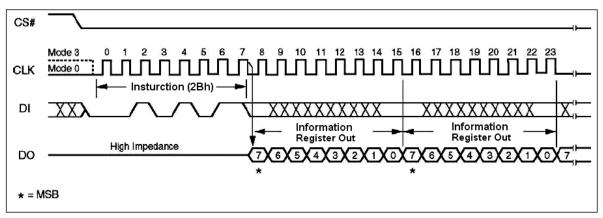
Figure 11. Read Information register Instruction Sequence Diagram
