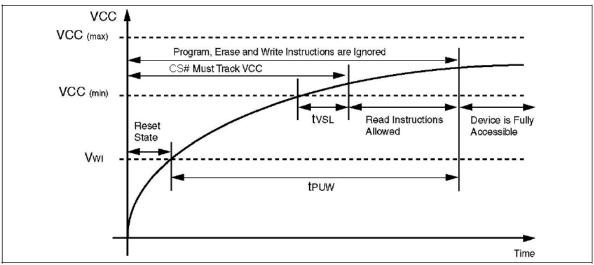
Figure 37. Power-up Timing
