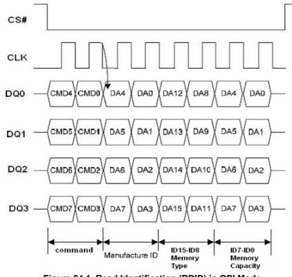
Figure 34.1. Read Identification (RDID) in QPI Mode
