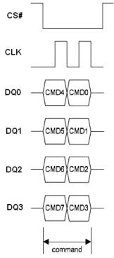
Figure 35.1 Enter OTP Mode Sequence under EQPI Mode
