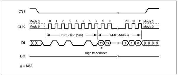
Figure 27. 32KB Half Block Erase Instruction Sequence Diagram
