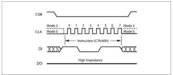
Figure 29. Chip Erase Instruction Sequence Diagram
