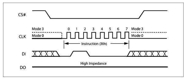
Figure 24. Write Resume Instruction Sequence Diagram
