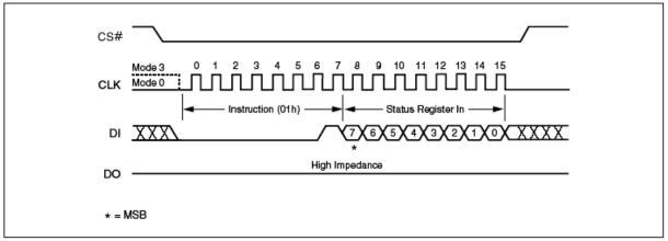
Figure 12. Write Status Register Instruction Sequence Diagram
