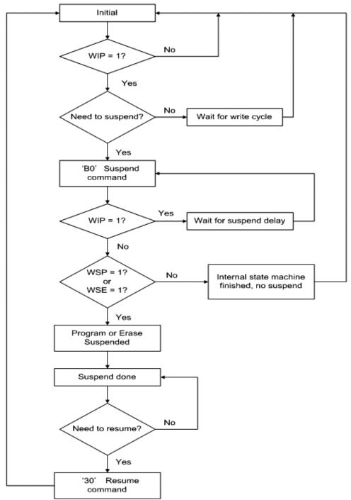
Figure 25. Write Suspend/Resume Flow
