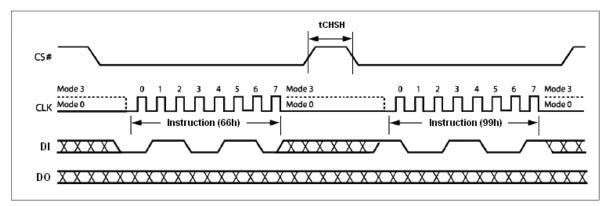
Figure 7. Reset-Enable and Reset Sequence Diagram
