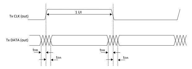
Figure 3.9. Transmit TX.CLK.Aligned Waveforms
