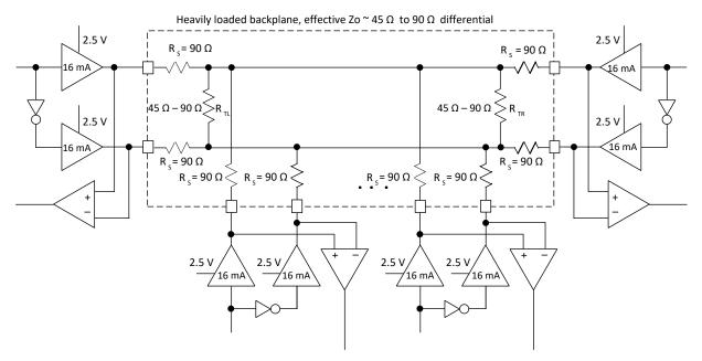
Figure 3.2. BLVDS25 Multi-point Output Example
