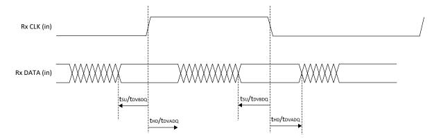
Figure 3.6. Receiver RX.CLK.Centered Waveforms
