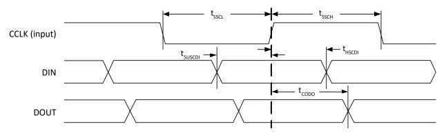
Figure 3.17. sysCONFIG Slave Serial Port Timing
