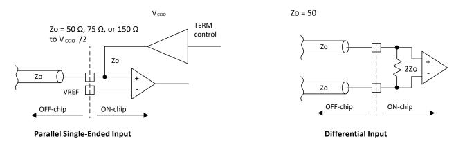
Figure 2.26. On-Chip Termination
