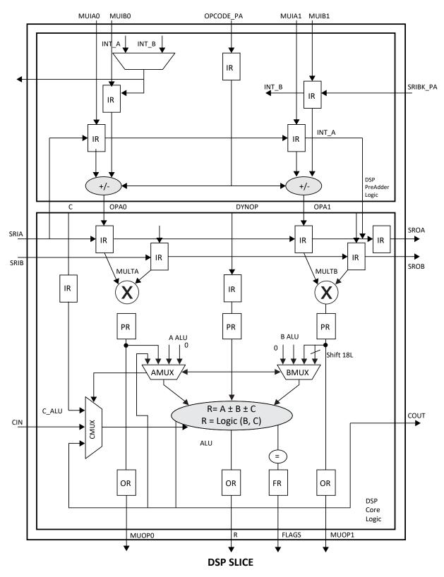
Figure 2.15. Detailed sysDSP Slice Diagram
