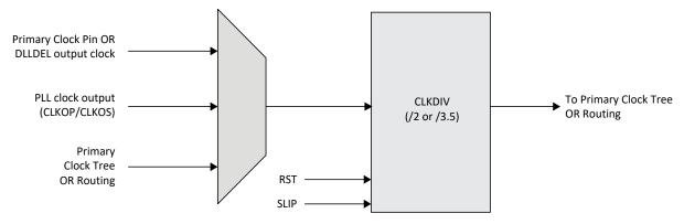
Figure 2.9. ECP5/ECP5-5G Clock Divider Sources
