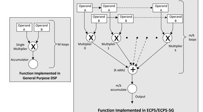
Figure 2.13. Comparison of General DSP and ECP5/ECP5-5G Approaches
