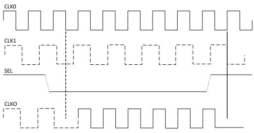
Figure 2.7. DCS Waveforms
