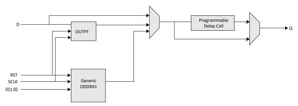
Figure 2.19. Output Register Block on Top Side
