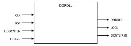
Figure 2.10. DDRDLL Functional Diagram
