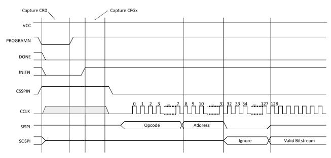
Figure 3.22. Master SPI Configuration Waveforms
