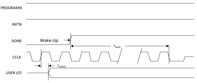
Figure 3.21. Wake-Up Timing
