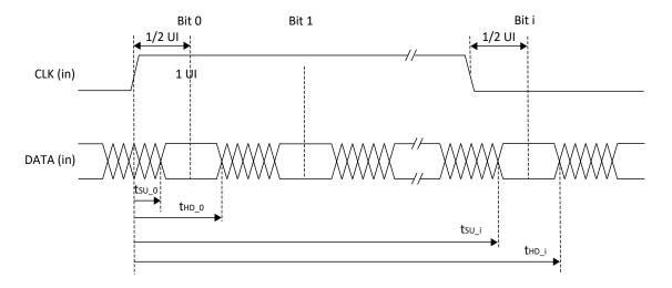
Figure 3.11. Receiver DDRX71\_RX Waveforms
