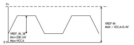
Figure 3.14. SerDes External Reference Clock Waveforms
