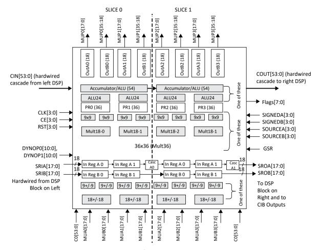
Figure 2.14. Simplified sysDSP Slice Block Diagram
