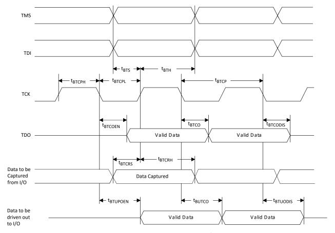
Figure 3.23. JTAG Port Timing Waveforms
