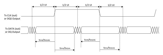
Figure 3.8. Transmit TX.CLK.Centered and DDR Memory Output Waveforms
