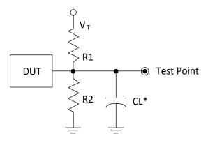
\*CL Includes Test Fixture and Probe Capacitance
