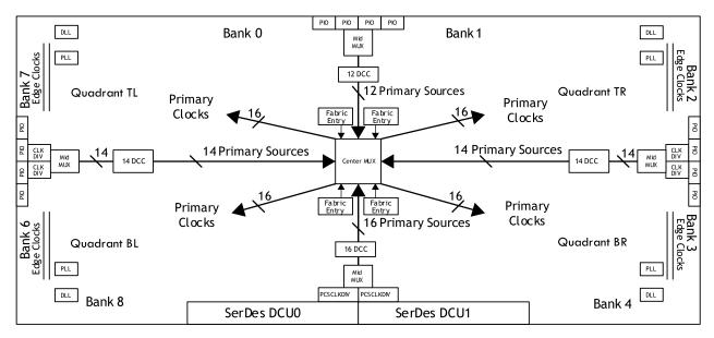
Figure 2.6. LFE5UM/LFE5UM5G-85 Clocking
