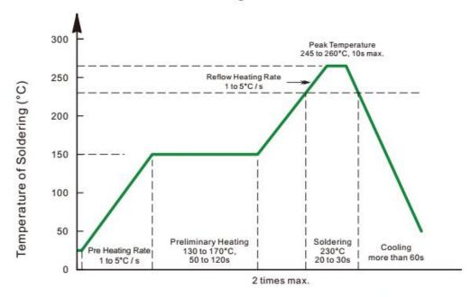
Recommended peak temperature is over 245 °C. If peak temperature is below 245 °C, you may adjust the following parameters; time length of peak temperature (longer), time length of soldering (longer), thickness of solder paste (thicker)
