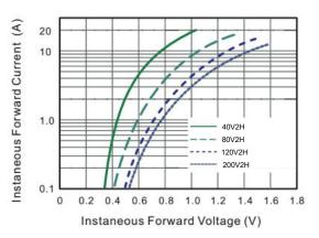
Fig.3 Typical Forward Characteristic
