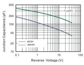
Fig.4 Typical Junction Capacitance
