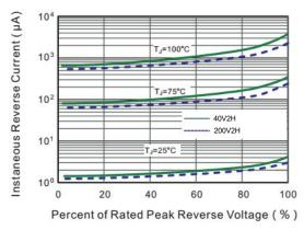
Fig.2 Typical Reverse Characteristics
