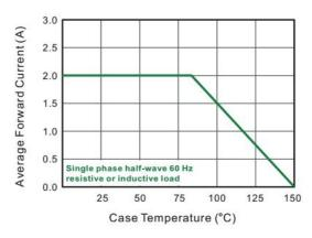
Fig.1 Forward Current Derating Curve
