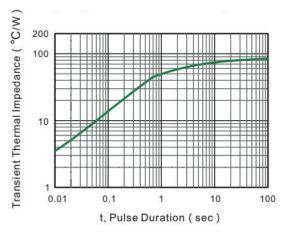
Fig.6 Typical Transient Thermal Impedance
