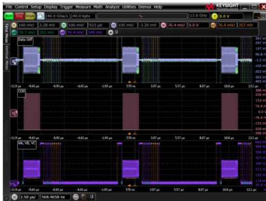
Figure 63 C-PHY Eye Pattern Example, Triggered Eye
