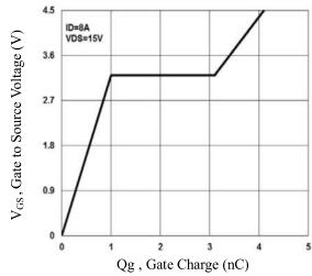
Fig.4 Gate Charge Waveform
