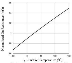
Fig.2 Normalized RDSON vs. T<sub>J</sub>
