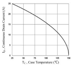
Fig.1 Continuous Drain Current vs. T<sub>c</sub>
