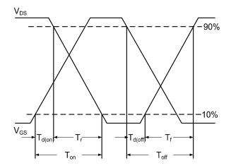
Fig.7 Switching Time Waveform
