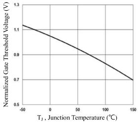
Fig.3 Normalized V<sub>th</sub> vs. T<sub>J</sub>
