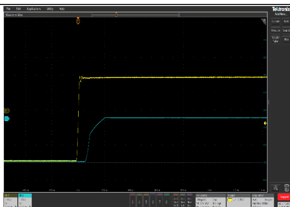
Figure 9. Step Response, V_{IN} = 5\text{ V} , C_{IN} = 1\text{ }\mu\text{F} , C_{OUT} = 1\text{ }\mu\text{F} , 200 \mu\text{s/div}
