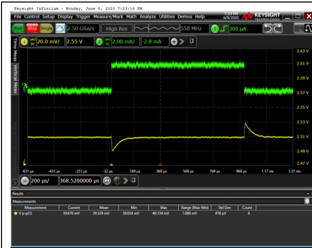
Figure 13. Load Transient, \pm 2\text{ mA} , V_{IN} = 5\text{ V} , C_{IN} = 1\text{ }\mu\text{F} , C_{OUT} = 1\text{ }\mu\text{F} , 20 mV/div
