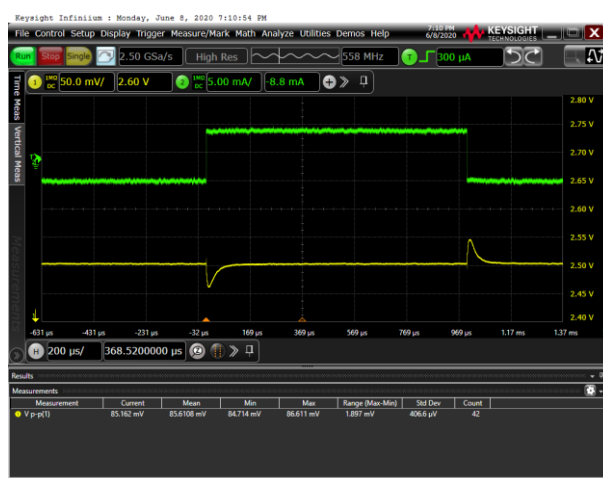
Figure 11. Load Transient, \pm 5\text{ mA} , V_{IN} = 5\text{ V} , C_{IN} = 1\text{ }\mu\text{F} , C_{OUT} = 1\text{ }\mu\text{F} , 50 mV/div
