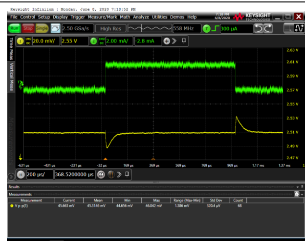
Figure 14. Load Transient, \pm 2\text{ mA} , V_{IN} = 2.8\text{ V} , C_{IN} = 1\text{ }\mu\text{F} , C_{OUT} = 1\text{ }\mu\text{F} , 20 mV/div
