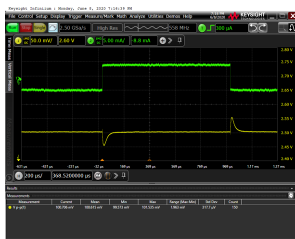
Figure 12. Load Transient, \pm 5\text{ mA} , V_{IN} = 2.8\text{ V} , C_{IN} = 1\text{ }\mu\text{F} , C_{OUT} = 1\text{ }\mu\text{F} , 50 mV/div
